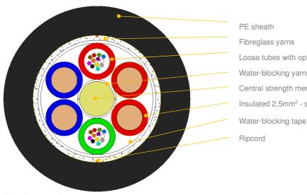
Loose tubes with optical fibres (PBT)
